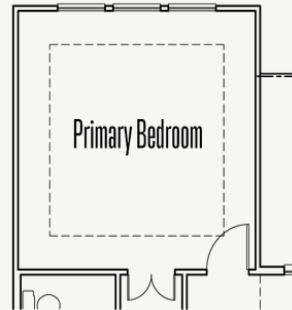
Optional Step Ceiling Treatment at Primary Bedroom
